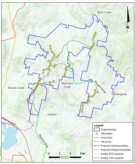
Bowmans Creek Wind Farm proposed site layout – the project involves 56 wind turbines and associated infrastructure connected to existing powerlines.
