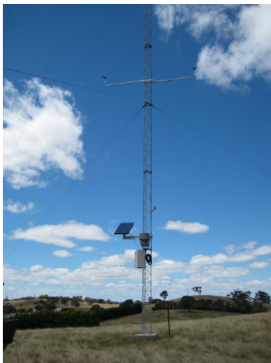
Wind Monitoring Mast (Solar Powered)
