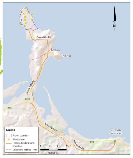
Western Plains Wind Farm - the proposed design involves 12 wind turbines connected to the Port Latta substation via a new underground powerline.
