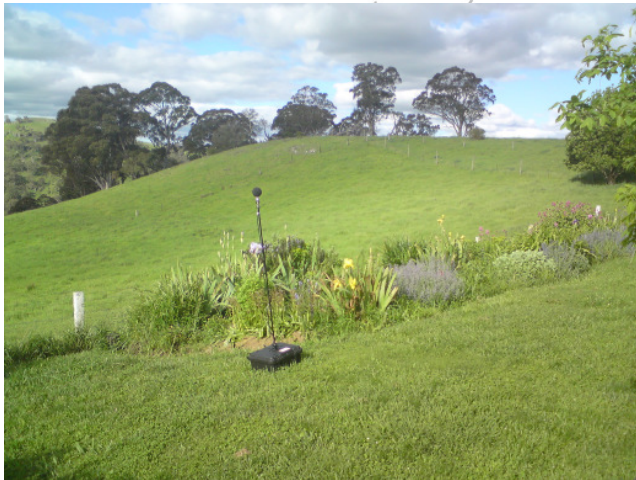
Noise loggers set up near associated residences, as per the Noise assessment requirements Epuron must undertake as part of the EA process.
