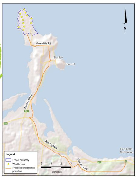
Map above shows the proposed layout of 12 wind turbines at the tip of the Stanley peninsula, connected to Port Latta Substation via a new underground powerline.
