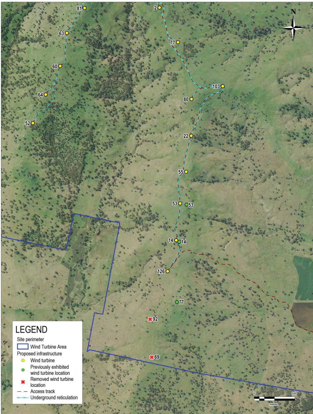
Figure 6-2: Example of change to wind turbine layout
