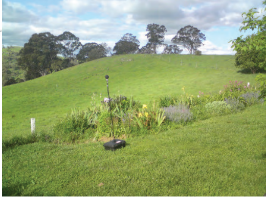
Noise data logger used to record background noise measurements at house locations around the wind farm site
