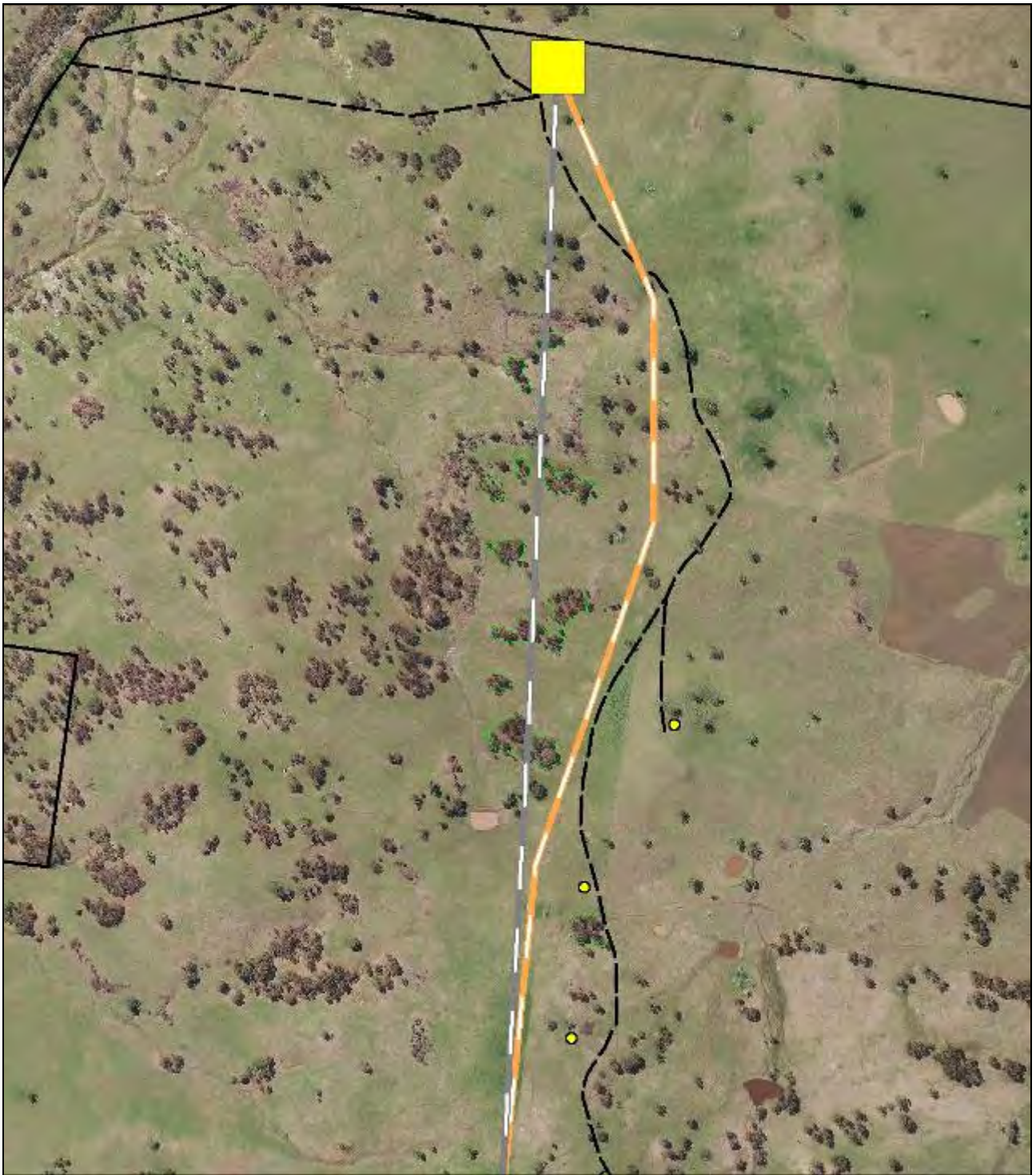
Plate 3: Example of relocated transmission line to avoid Yellow Box EEC. Grey – original transmission line location. Orange – relocated transmission line.
