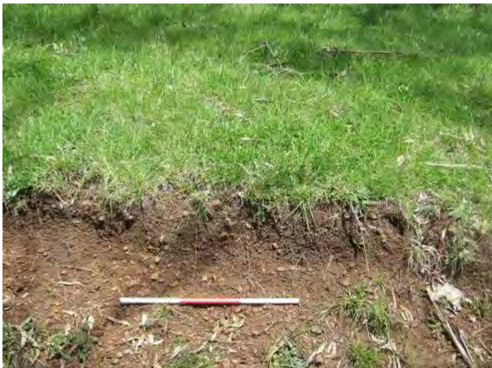
Plate 10 Survey Unit 2 shallow topsoil 20-30 depth underlain by weathering basalt (orange fragmented rock).
