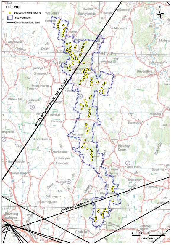
Figure 4-2 Point to point radio communication links in the vicinity of the Rye Park Wind Farm (Revised turbine layout)
