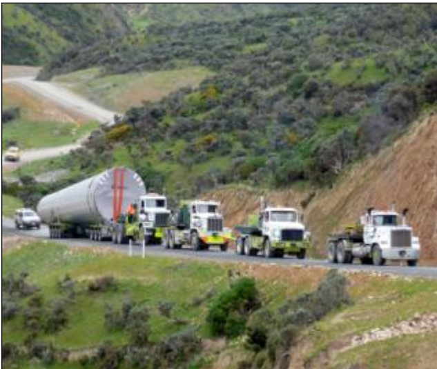
Figure 6-2 Transport of tower section on steep site access track
