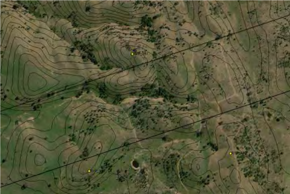
Figure 5-4 – Zoomed-in aerial showing moved locations of turbines in yellow, now outside of the Fresnel zone.
