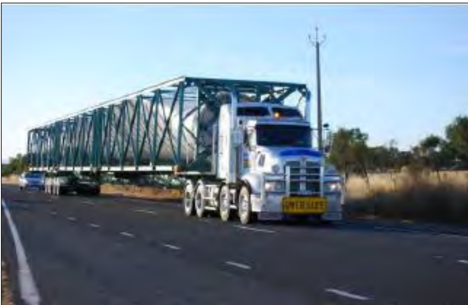
Figure 6-1 Transport of turbine blades with escort vehicle
