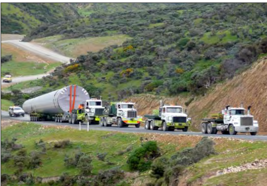
Figure 6-2 Transport of tower section on steep site access track
