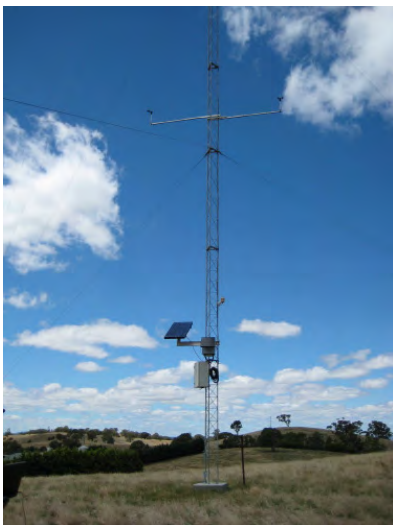
Wind Monitoring Mast (Solar Powered)
