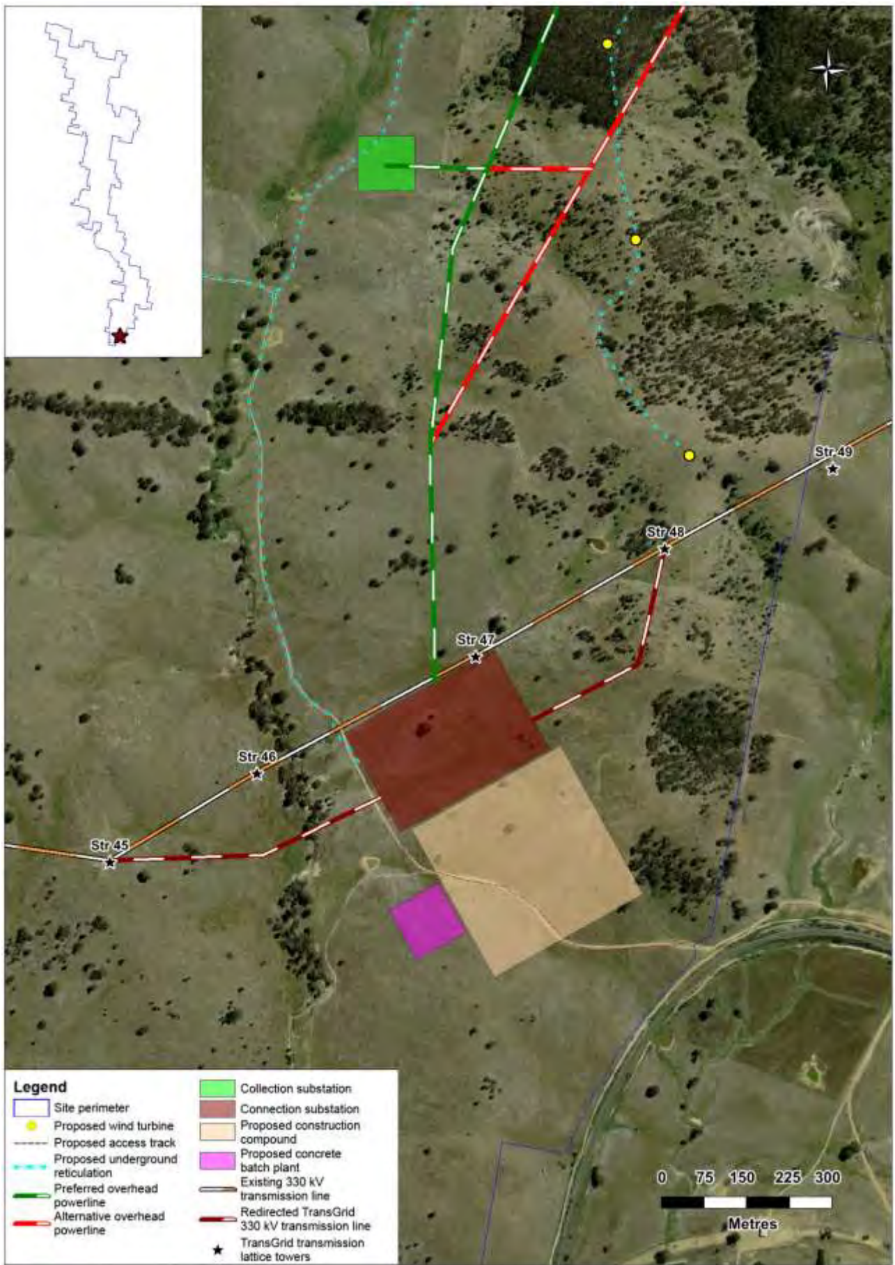
Figure 3-22 Proposed wind farm connection substation, southern construction compound, line deviation route and concrete batch plant
