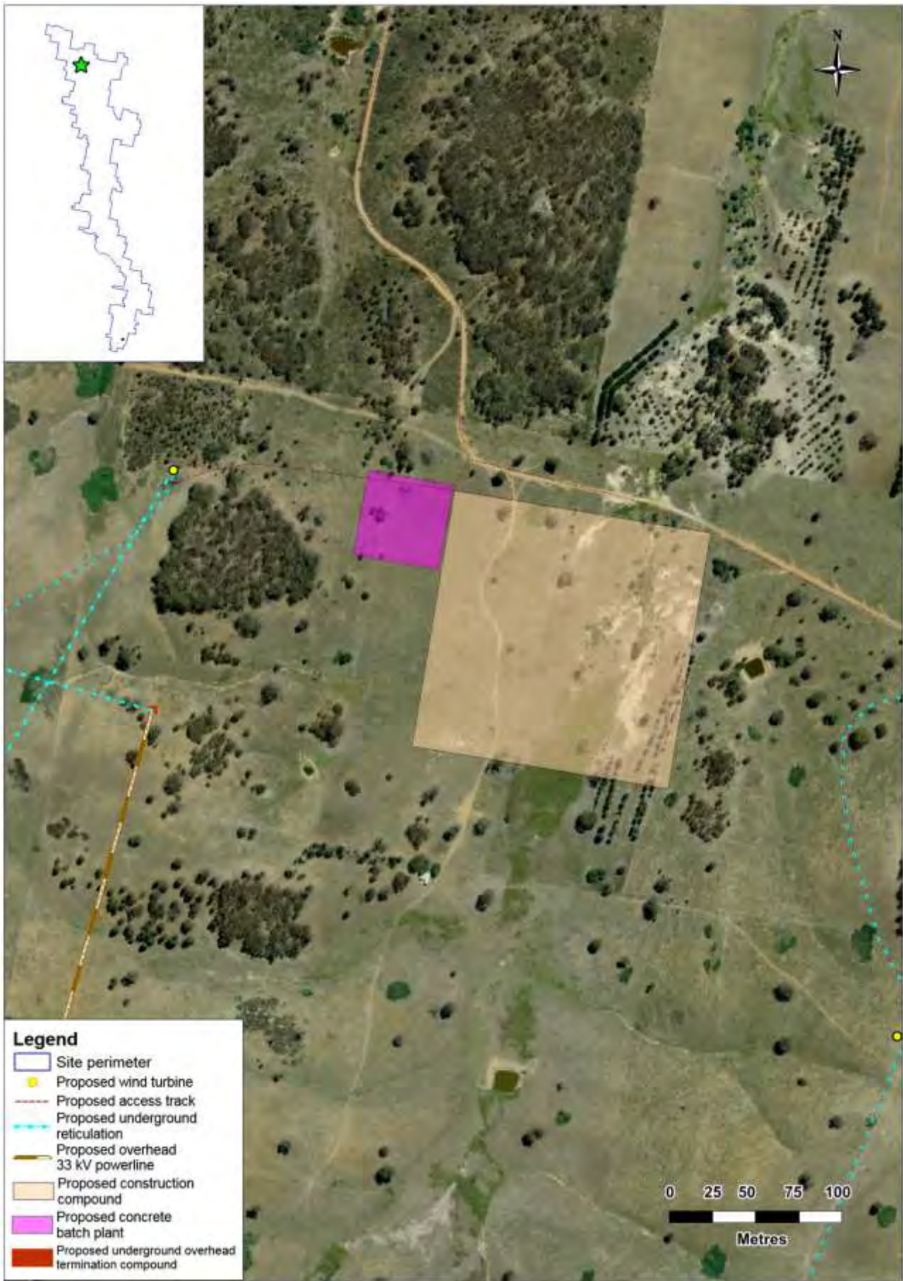
Figure 3-23 Proposed northern construction compound and concrete batch plant
