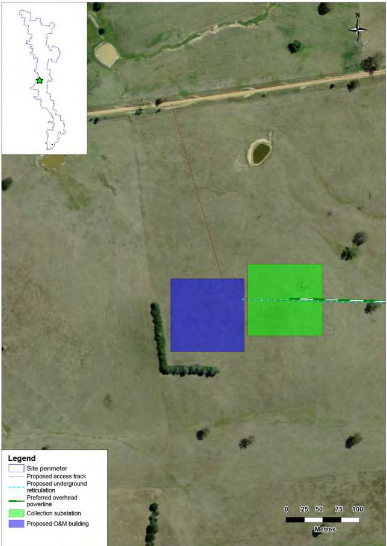
Figure 3-21 Proposed central wind farm collection substation and permanent operation and maintenance facility
