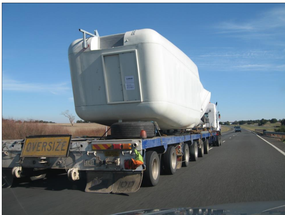
Figure 2-1 Transport of wind turbine nacelle
