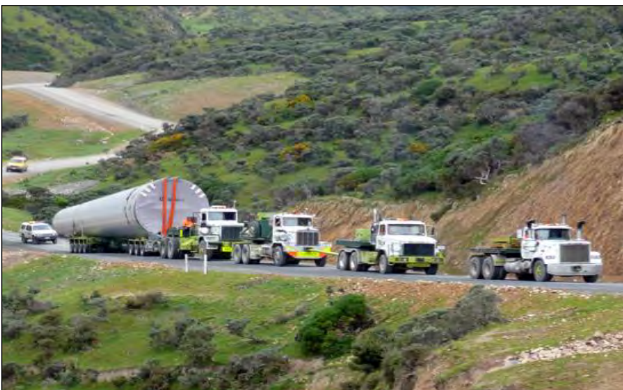
Figure 6-2 Transport of tower section on steep site access track
