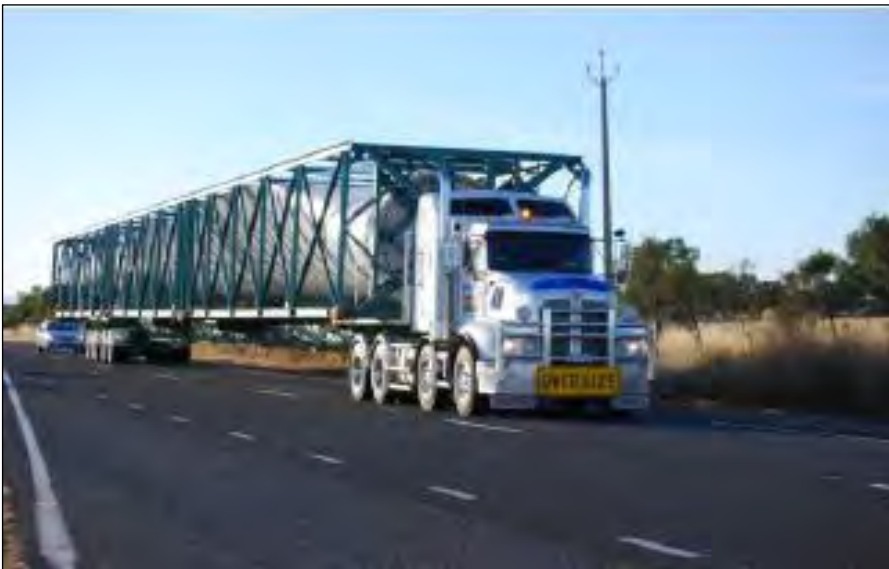
Figure 6-1 Transport of turbine blades with escort vehicle
