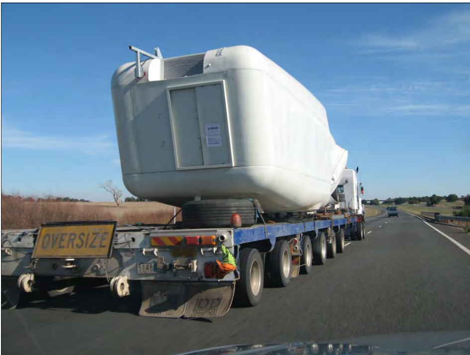
Figure 2-1 Transport of wind turbine nacelle
