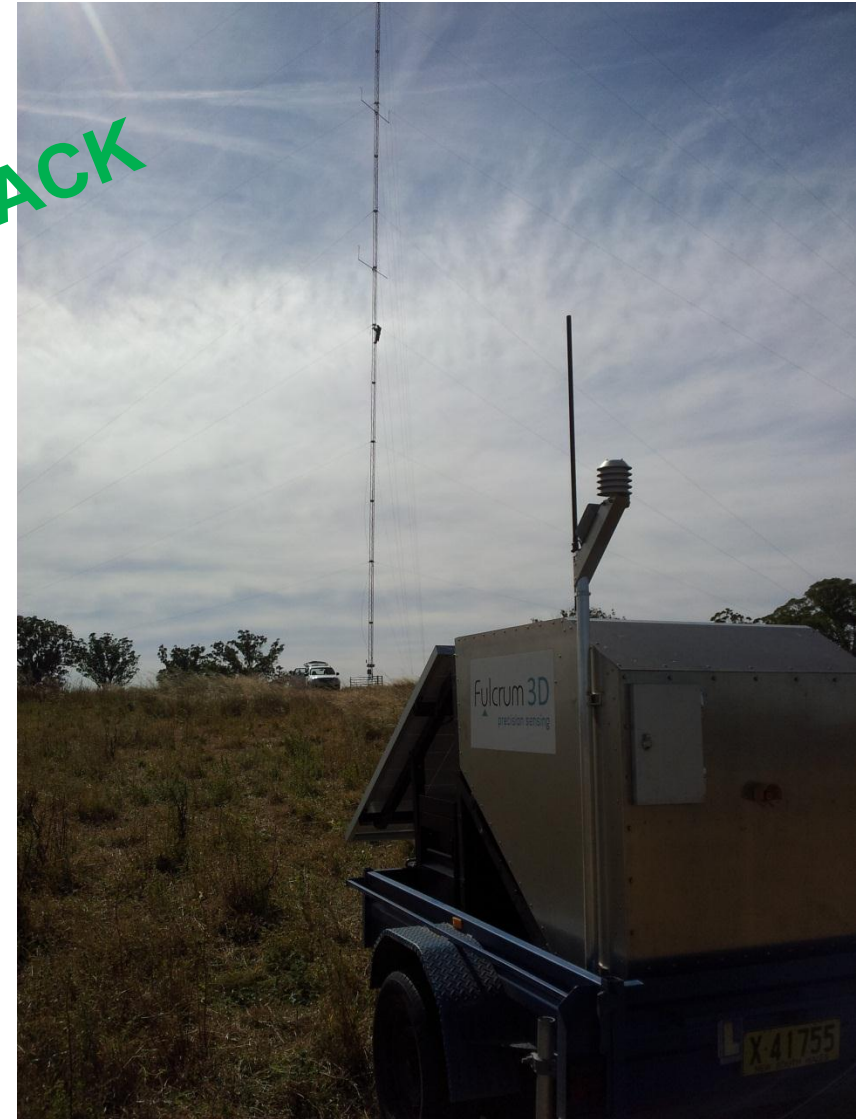
Liverpool wind monitoring mast and Sodar
