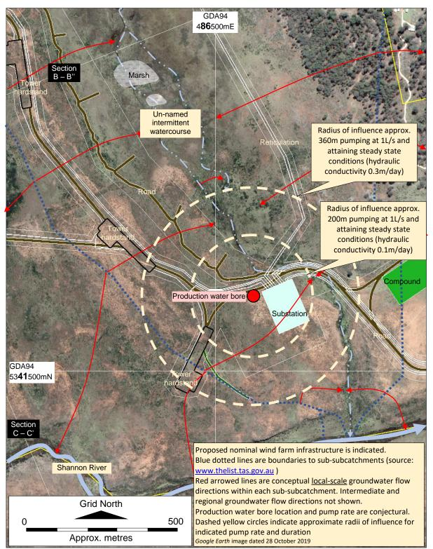
Figure 15. Inferred local-scale flow directions and proposed (nominal) wind farm infrastructure near the Shannon River on St Patricks Plains. Also shown as an example are the radii of influence of a hypothetical production water bore for two different hydraulic conductivities, under steady state conditions and pumping at 1L/s. The thickness of the fractured, unconfined dolerite aquifer is assumed to be 50m.
