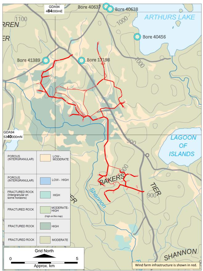
Figure 8. Published prospectivity of the fractured rocks and unconsolidated alluvium in the vicinity of the proposed St Patricks wind farm.
