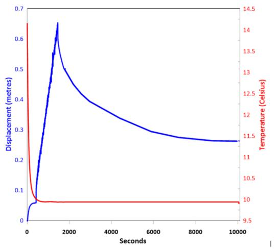
Figure 9. Time series water level and temperature data for the pump test of bore 17198.
