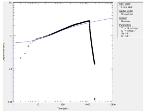
Figure 12. Time series displacement pumping of bore 41389.
