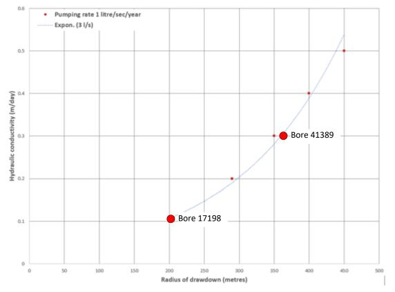
Figure 13. Maximum radii of influence for different hydraulic conductivities in the unconfined dolerite aquifer in the vicinity of the proposed St Patricks Plains wind farm. This graph is based on pump testing the only two operating bores in the district. Different hydraulic conductivities are very likely to be obtained from bores drilled in other locations in the same dolerite aquifer, so the graph should be regarded as indicative only.
