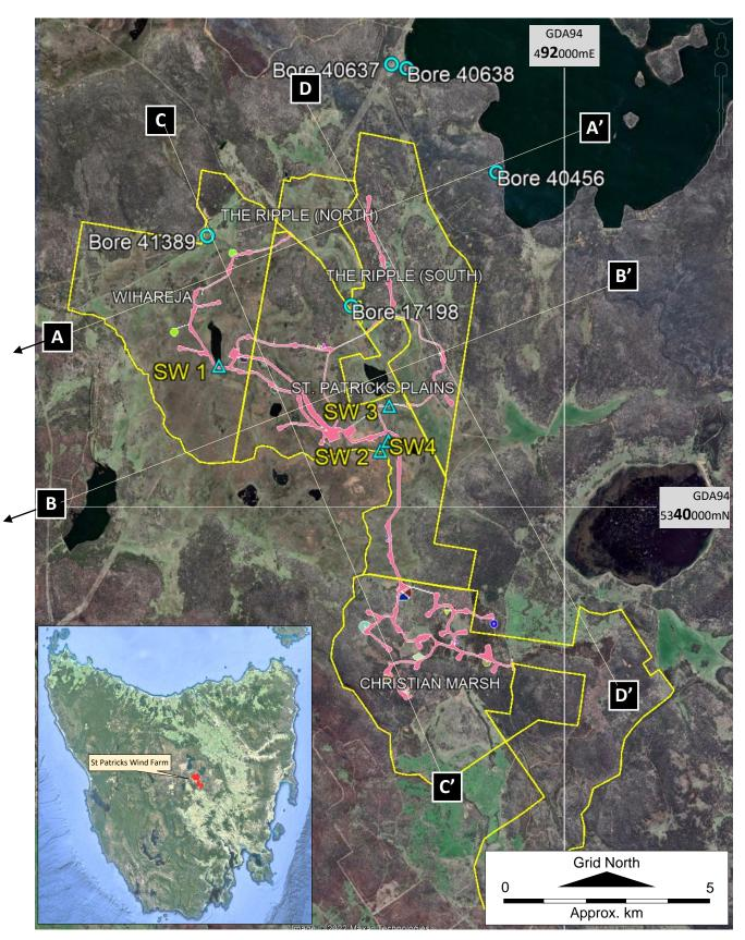
Figure 2. St Patricks wind farm infrastructure (pink lines) on St Patricks Plains. Yellow lines are property boundaries. Also shown are hydrogeological cross section lines A – A'.....D – D'. Recorded groundwater bores (Bores 41389 and 17198) were pump tested and sampled for this report, and surface water locations SW1, SW2, SW3, SW4 were sampled for this report) Source of base image: Google Earth; image date 28 October 2019.
