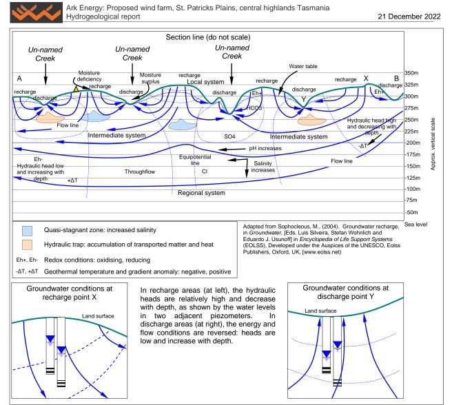
Figure 5. Fundamentals of groundwater hydrology in a gravity-driven groundwater system like that in the study area. Vertical exaggeration for the top section is about 5.
