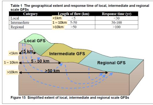
Figure 6. The conceptual sizes of, and travel times for groundwater through, local-. Intermediate- and regional-scale GFS's. The sizes of each GFS for the study area are shown at left, and the travel times in the left centre of the table.
