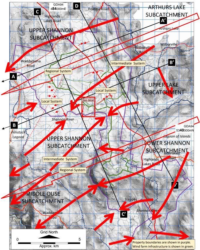
Figure 7. Inferred groundwater flow systems (GFSs) in the vicinity of the proposed St Patricks Wind Farm. Open arrows are regional GFSs; solid red arrows are intermediate GFSs; thin red arrows are local GFSs. Hillshade image: <a href="https://www.thelist.tas.gov.au">www.thelist.tas.gov.au</a>
