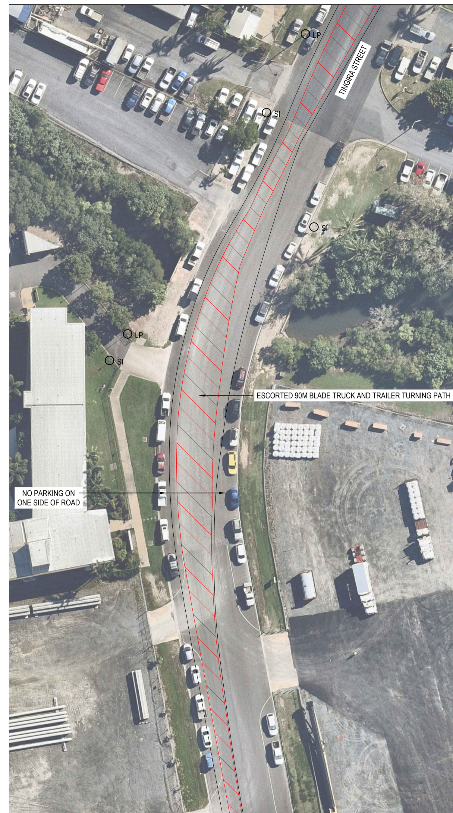
TINGIRA STREET BEND - 90m BLADE TRUCK AND TRAILER (TRAVELLING TO SITE)
