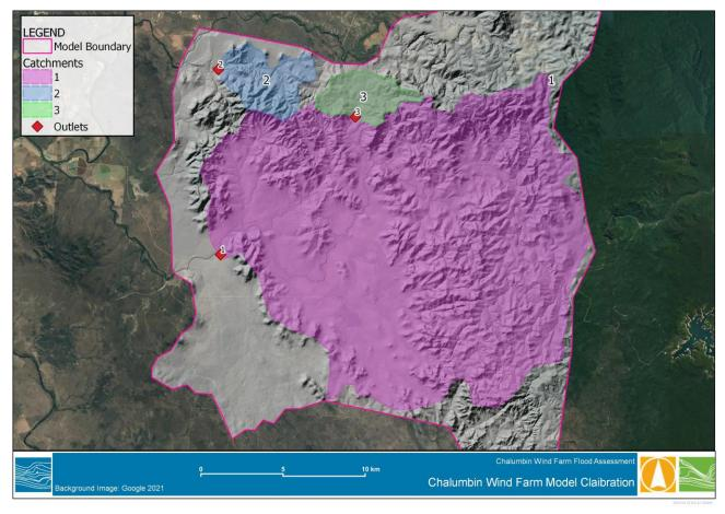
FIGURE 6 DELINEATION OF CATCHEMNTS USED FOR MODEL VALIDAITON
